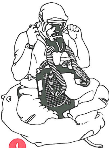
4 PUT ON OXYGEN MASK, TURN ON OXYGEN SYSTEM
